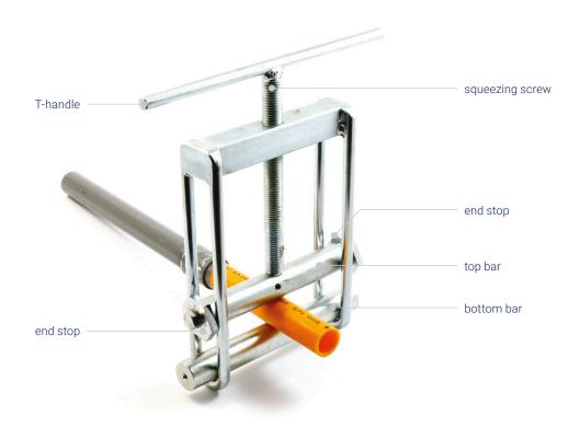
A manual screw pipe squeeze-off tool allows you to manually clamp polyethylene pipes to temporarily shut off the flow of medium inside a pipeline. When using the tool, follow the health and safety rules.
